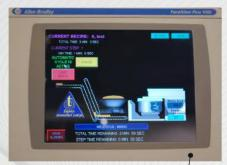
Fully graphic operator touch screen for automated control and status indications. When used without the dough chunker-elevator, the dough can be deposited onto a mobile table or into a mobile fermentation trough as desired.
